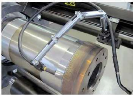
External Overlay welding
