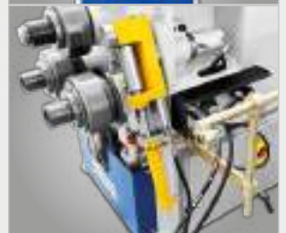
▶ Option: hydraulic straightening rollers
