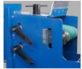
▶ Easy height adjustment of grinding belt without tools
