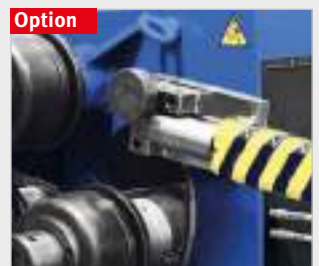
▶ Option: two lateral hydraulic guide rollers
