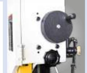
▶ Saw band guide height-adjustable via hand wheel
