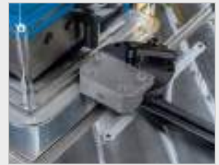
▶ Stops with adjustable blank holders
