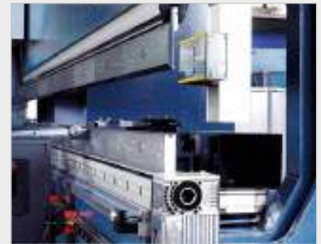
► Hydraulic tool clamping (option)
