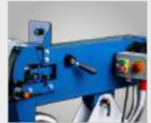
Tension/relieve belt via lever
