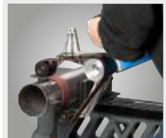
Only two work steps necessary for 360° circumference grinding
