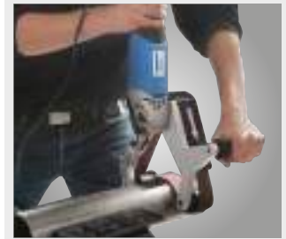
Handle for ergonomic work can be screwed in at various positions
