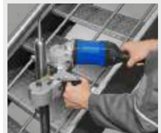
Pivoting grinding arm for optimum adjustment to the required grinding position
