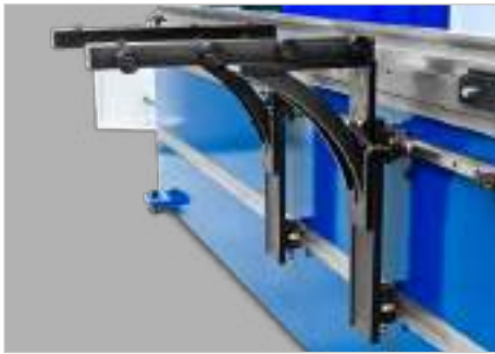
► Sheet support arms displaceable on linear rails
