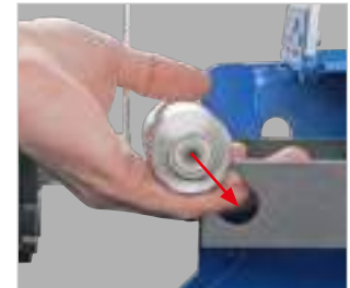
▶ Thanks to the optimised quick-release holder, the grinding roller can be easily and quickly replaced without tools
