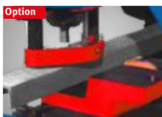
▶ Optional die block for U sections
