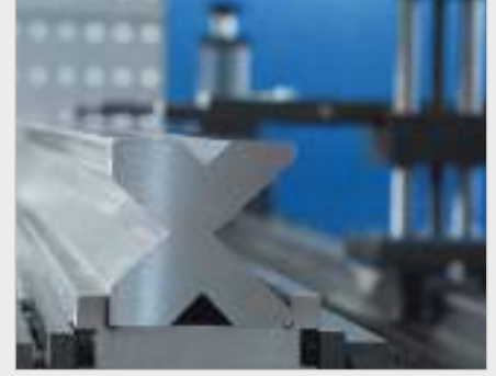
► Standard centring rail with optional, tempered and polished Multi-V die
