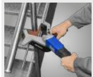
Especially suitable for processing installed railings
