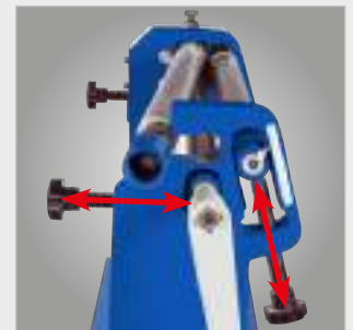
▶ Rear rollers individually adjustable, thus supports conical work ▶ Settings through convenient, generously dimensioned roller adjustment screws
