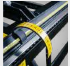
▶ Scale shows bending angles from 0 - 120°
