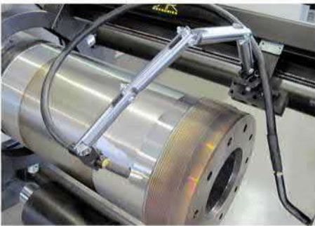
External Overlay welding
