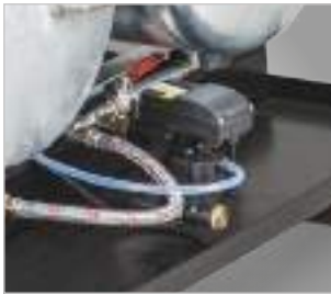
· Automatic condensate drain on vessel
