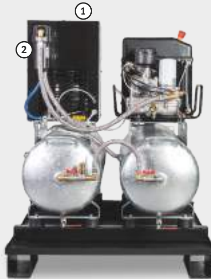
DUO K equipment 1. Refrigeration dryer with integrated automatic condensate drain, pressure dew point 5 °C, compressed air inlet temperature 35 °C, cooling air temperature 25 °C 2. Fine filter as prefilter upstream of the refrigeration dryer for separating condensate and solid contamination with a particle size of up to 1 µm (compressed air quality as per ISO 8573-1)
