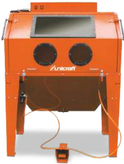
Fig. shows SSK 3.1 featuring a very large front flap which opens upward
