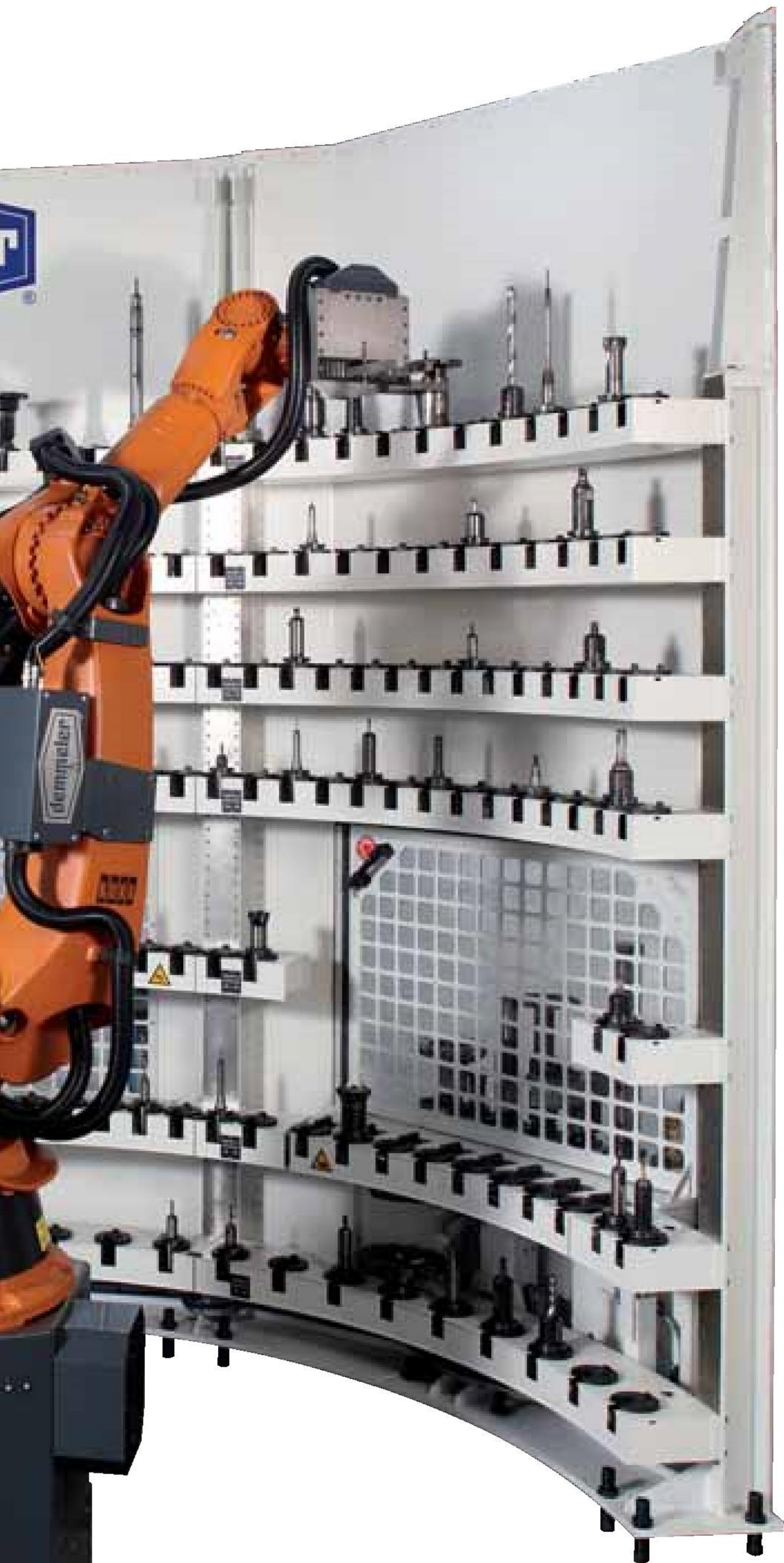
6-axis standard industrial robot as tool magazine and changer at production machines
