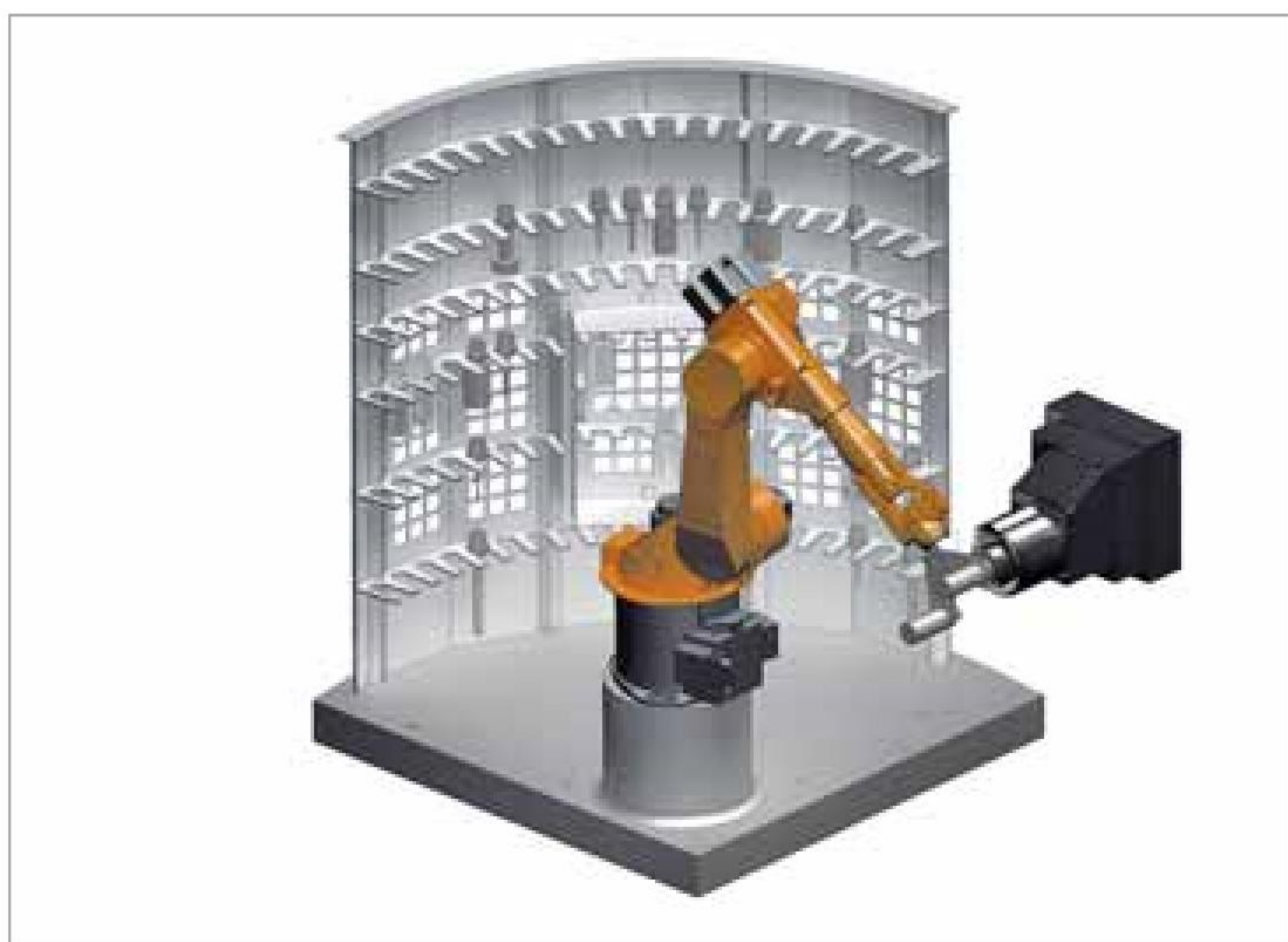
Horizontal tool change directly in machine spindle
